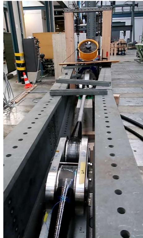
Fatigue experiments in 2020 on CFRP hangers
