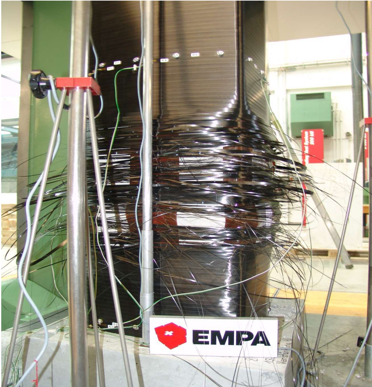
Externally Bonded FRP: Confinement
