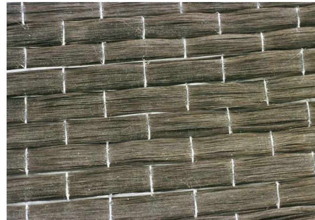
CFRP fabric (SikaWrap® Hex-230C)
