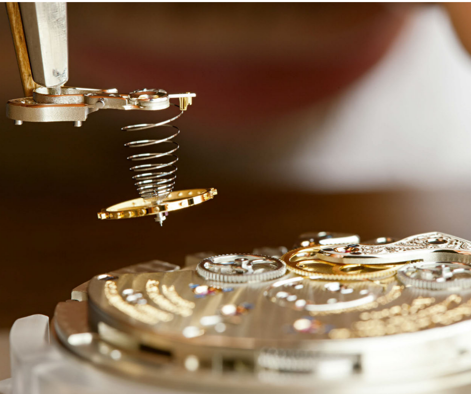
The balance wheel is the beating heart of every mechanical watch mechanism. The delicate springs are usually made of cast, forged Nivarox alloy. At Empa a new generation of balance springs is produced with means of electroplating.
